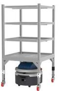
Use any web-enabled or integrated device such as Zebra tablets or mobile computers to execute a workflow or request a pick-up. Zebra Connect will automatically move to the pick-up area and autonomously transport it to the selected drop-off area. Upon arrival, Zebra Connect automatically detaches from the cart and is ready for the next task, keeping workers productive in their zones.
